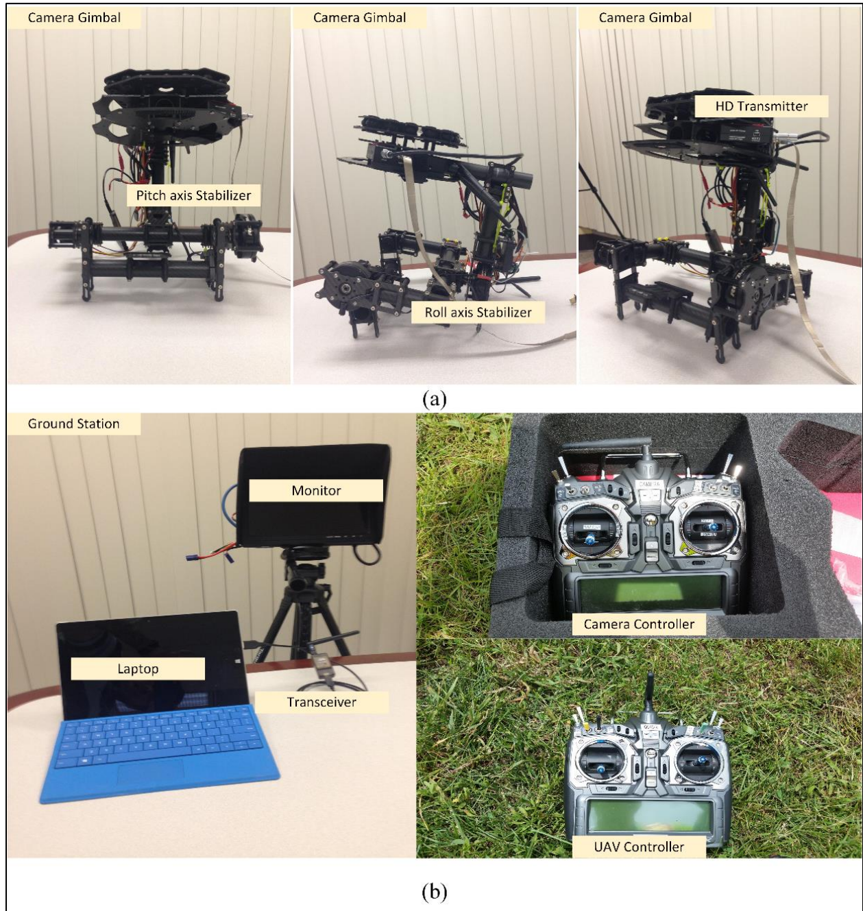
Figure 13. QU4DX UAS Components: (a) camera gimbal, and (b) ground station
