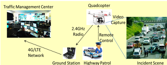
High-level Framework for Quadcopter-based Incident Monitoring
