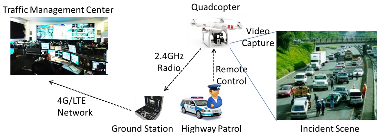
Figure 3 High-level Framework for Quadcopter-based Incident Monitoring
