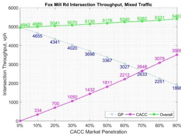
(a) Throughput at Fox Mill Rd intersection in mixed traffic deployment
